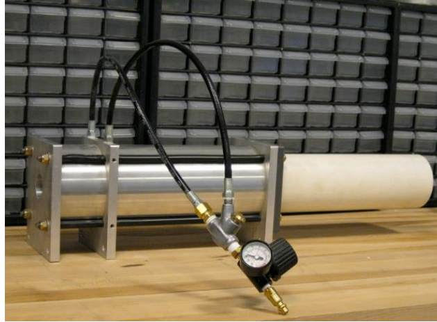
Figure 1.3 Shock tube of length 26 inches comprised of an aluminum exterior with vasiform exposure chamber.
