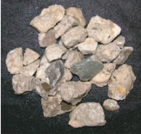
Figure 1.1 RCA particles with a large amount of adhered mortar [3].
